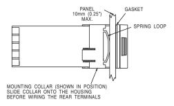
against the panel until the spring loops are slightly compressed. The ratchets will hold the mounting collar and housing in place.
