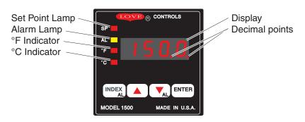
The °F/°C indicator will flash while Self-Tune is operating. The rightmost decimal point flashes while the ramping function is active.
