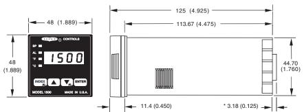
Panel cutout for all models is 45mm x 45mm (1.775 in x 1.775 in). Allow for 13 mm (0.5 in) clearance at the rear of the instrument.
